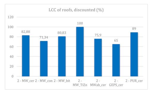
The most expensive roof is the MW-bit and MW-TiZn. Roofing with concrete tiles (MW\_con) is the most cost effective solution.
