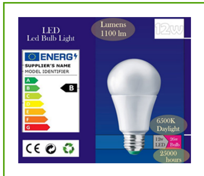
Figure 33: Information on packaging. (The efficacy is: 1100\text{lm}/12\text{W}=91\text{lm}/\text{W} )
